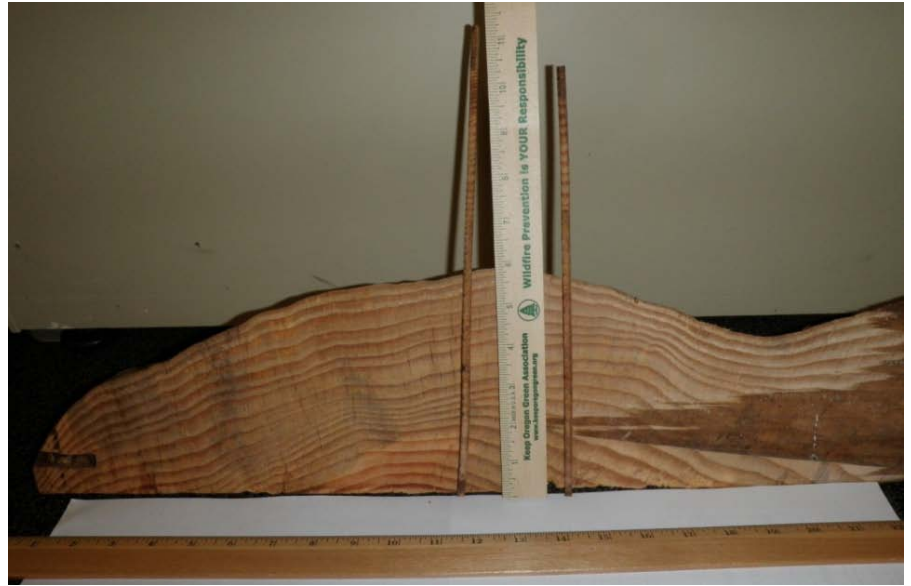
Figure 4: Douglas-fir, 44 inches DBH from Airstrip 7A, wedge and 2 cores (File photo by K. Walton, 2011, section 7, T4S. R5E)
